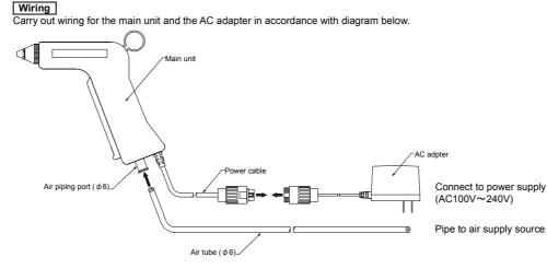
• Connect the power cable of a main unit to the AC adapter.
