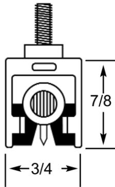
The BR2200 static bar is easily and conveniently mounted on the ends, and anywhere along its length, by using the weld screws that slide inside the channel on the opposite side of the emitter pins. This mounting method coupled with the ruggedness of the aluminum profile minimizes sag even over the longest lengths.
