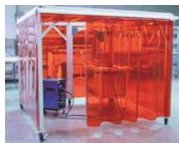
MACHINERY AND WELDING ENCLOSURES
