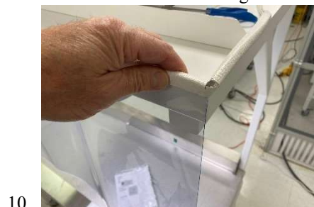
10. with the fascia flush at the right end of the ceiling, position the edging over the fascia and press a few inches of the edging down to retain the fascia laterally (left-to-right)
