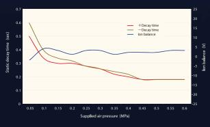
(Note 1) Using □150mm, 20pF charged plated monitor for measurements (Note 2) Static elimination time equals the decay time ±1000V→±100V (Note 3) ZappAURA 50mm from the plate monitor (Note 4) Using standard nozzle ANS
