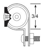
The BR2200 & BRE2200 static bars are easily and conveniently mounted on the ends, and anywhere along their length, by using the weld-screws that slide inside the channel on the opposite side of the emitter pins. This mounting method coupled with the ruggedness of the aluminum profile minimizes sag even over the longest lengths.
