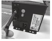
**IMPORTANT**: If the HV cable is higher than the Power Supply be sure to route the HV cable to have a dip or curve near the power supply so that any fluids that may leak or spill onto the cable drip from the cable rather than follow it into the HV socket of the Power Supply.
