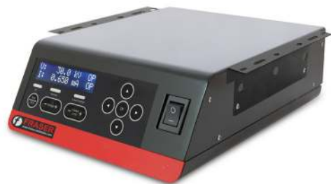
The brackets can be fitted to allow for "under bench" mounting.
