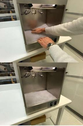
5. PLACE THE PERFORATED FLOOR INSIDE THE CHAMBER TO SIT ATOP THE FRONT AND REAR LIP AS SHOWN BELOW.
