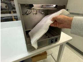
2. PLACE THE NEW PREFILTER SUPPORT WIREFRAME INSIDE THE CHAMBER, WITH THE TEARDROP EYELETTES OVER THE PEM NUT AND STUD AT THE FRONT OF THE CHAMBER FLOOR AS SHOWN BELOW. THIS WILL KEEP THE FRAME IN POSITION WHEN CHANGING THE PREFILTER PANEL.
