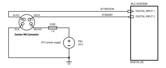
To interface the Ionizer with a PLC system having IEC 61131-2 Type 1 or Type 2 input characteristics, fit an external 1  $k\Omega$  pull-up resistor to supply the current required by these input types, as shown below. The resistor should have a power rating of at least 1 W.
