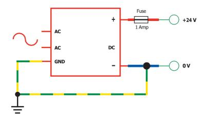
The 24 V supply connection (Pin 1, brown wire) **must be** fitted with a 1 A fuse. It is recommended that a type 'T' or 'G' fuse is installed.
