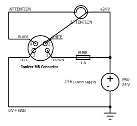
IMPORTANT: Connecting indicators with higher current requirements to the Ionizer will not damage it, but it is unlikely that satisfactory brightness will be obtained.
