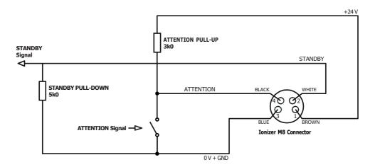
The switch in the diagram above is shown in the position corresponding to 'Ionizer powered, all  $\mathsf{OK}'$ .
